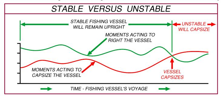
**Important Lesson** - The key to having a **stable** vessel is making sure there is sufficient stability to counter the capsizing moments from the current weather, waves, and fishing conditions during the **entire** voyage.
