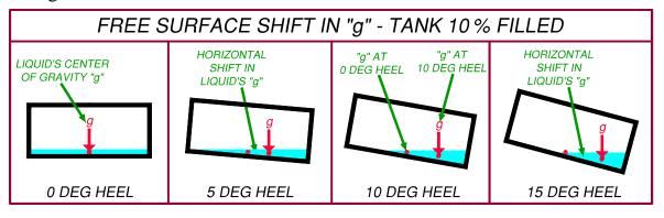
This shift in the liquid's center of gravity "g" causes the vessel's center of gravity "G" to shift outboard, reducing the righting arm "RA" as shown in the figure to the right.
