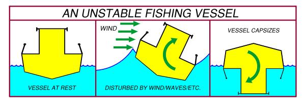
A fishing vessel is called **unstable** when it does not have enough positive stability to counter the external forces generated by <u>current</u> weather and fishing conditions and capsizes.
