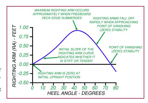
The shape of the righting curve at low angles of heel indicates how the vessel responds when subjected to low to moderate wind and waves.
