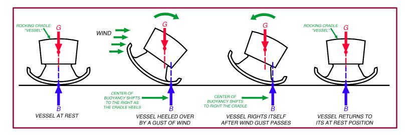
As with a fishing vessel, the cradle's (vessel's) center of gravity "G" is above its rocker, the center buoyancy "B". The slightest disturbance (wind, waves, or the movement of weight on the deck) causes the cradle (vessel) to roll (heel) to one side.
