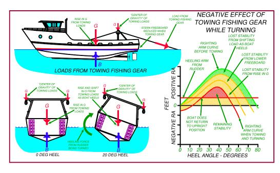
Fourth, the rudder creates a heeling moment (shown as the red line "Heeling Arm" in the figure), further acting to capsize the vessel.
