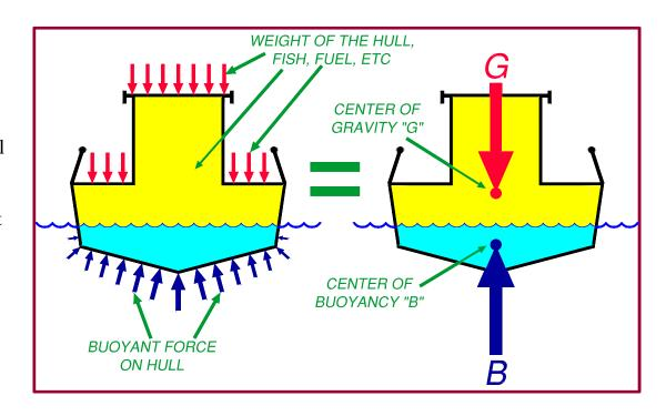
**Buoyancy** is the force acting to push the vessel up in the water; making the vessel float. In stability analysis, the total buoyancy forces, which are distributed over the part of the hull below the water, are mathematically combined into a single point called the Center of Buoyancy. This point is labeled "B" on stability model diagrams.
