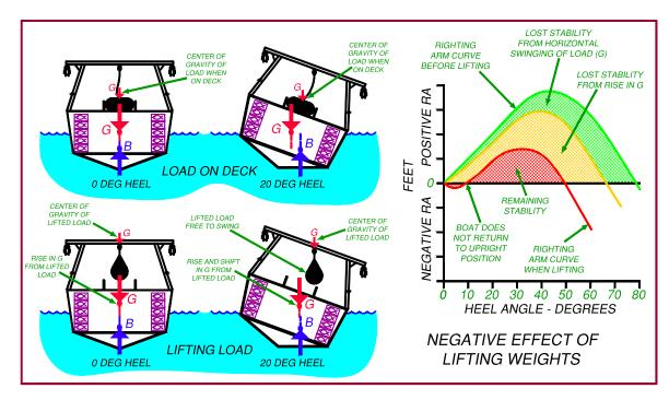
Recommendations: Never lift more weight than recommended in the vessel's stability guidance.
