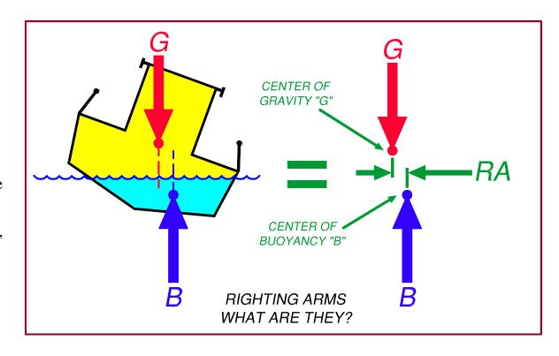
When the center of buoyancy "B" has shifted farther outboard than the center of gravity "G" as shown in the figure, the righting arm "RA" is a positive number creating positive stability.
