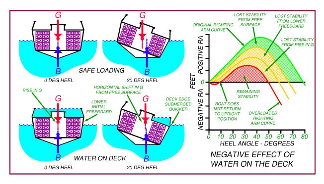
Because the trapped water on deck is located high on the vessel, the fishing vessel may not return to the upright equilibrium condition. Instead, it will lay over or "loll" at the angle of heel where the new righting arm curve goes through zero.
