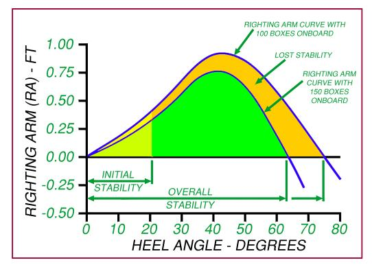
There is a potential hidden danger in using a fishing vessel's "feel" to determine if the vessel is safe from capsizing. The initial stability felt by the crew can be deceiving and give a false impression that the vessel has adequate stability levels. It may be too late to correct a problem by the time the vessel "feels" unsafe.
