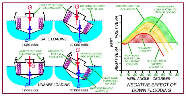
After downflooding occurs, the vessel's overall stability is reduced because:
