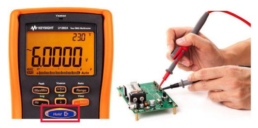
**Figure 5.** Hold & Export button—one press for three actions: Measure, save it into handheld DMM's memory and send the measurement out via infrared port. Optional U5404A remote switch probe emulates 'Hold & Export' button.
