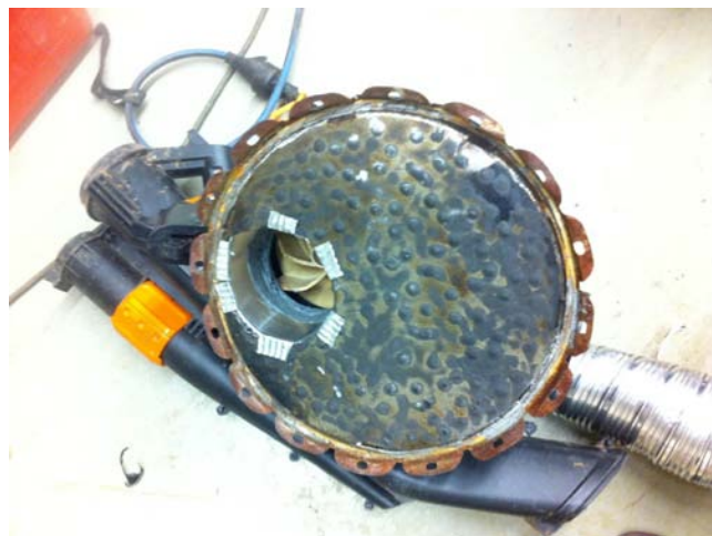
Figure 7. The lid used to seal the filter system with dryer outlet inserted to hook up the blower unit. The unit is also sealed with high temperature caulking.
