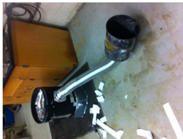
Figure 8. Completed gasifier unit connected to the filter system using dryer hose attached to two dryer outlets and sealed with metallic duct tape.
