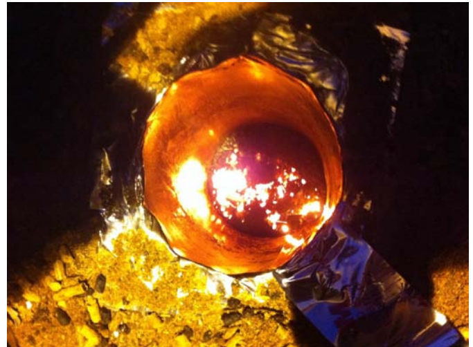
Figure 14. Top view of the fire inside the fire tube at the beginning before filling with the fuel source.
