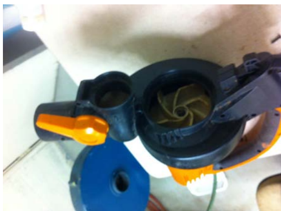
Figure 5. Blower unit used to create the down draft inside the gasifier before it was incorporated into the system.
