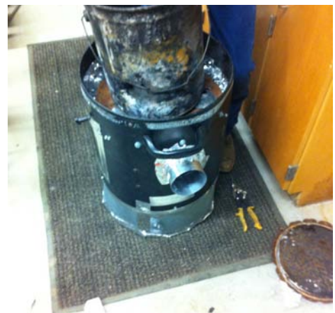
Figure 3. Construction of filter unit (five gallon bucket with outlet in bottom). The bottom part is the gasifier unit.
