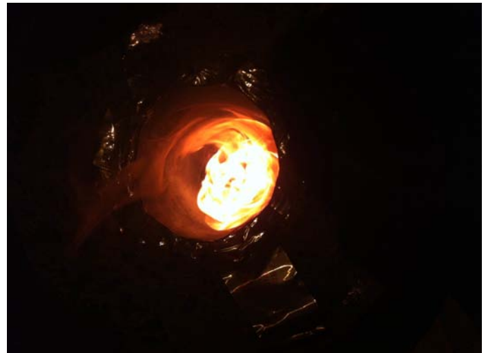
Figure 15. Top view of fire tube. Flame created if you do not turn the blower on to create the down draft.
