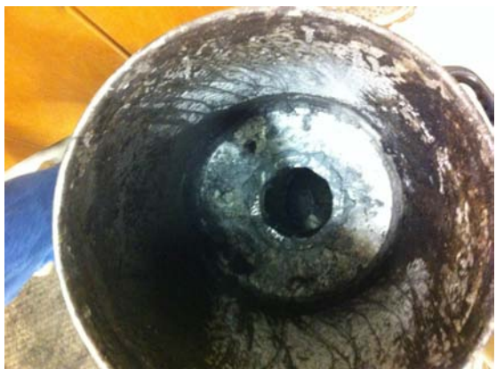
Figure 4. The inside of the filter unit (five gallon bucket) with dryer outlet attached. Inserted in the bottom and sealed with high temperature caulking.
