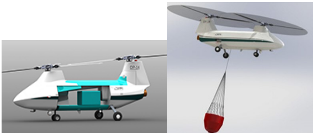
Figure A4. The DP-14 configured for internal and external cargo.
