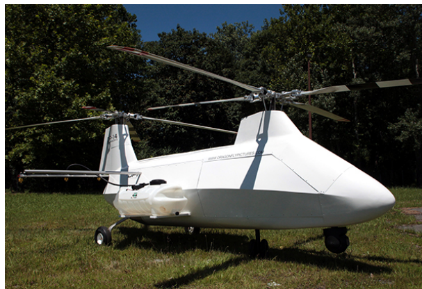
Figure 2. Dragonfly Pictures' DP-14 Model UAS Configured for Precision Aerial Application
