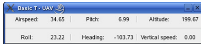
Figure 33 - Basic T monitoring window.
