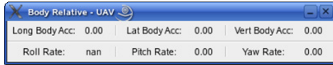
Figure 36 - Body Relative states monitoring window.
