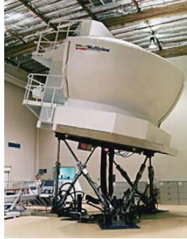
Figure 3 - Advanced Concepts Flight Simulator (ACFS).
