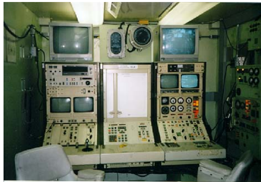
Figure 4 - Pioneer UAV Ground Control Station.
