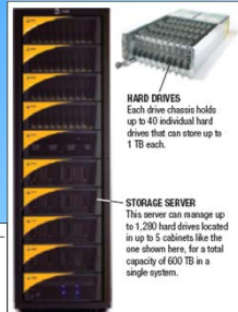
FIGURE 3-22 Storage servers. Storage servers are usually available so additional hard drives can be added as needed.
