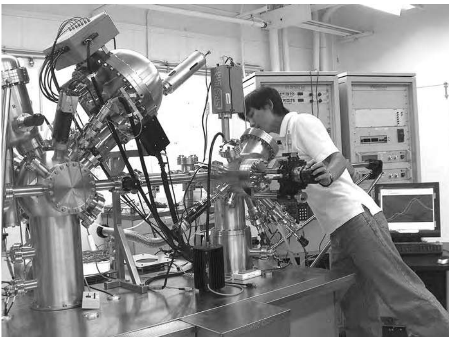
The X-ray Photoemission Spectrometer and UV Photoemission Spectrometer is equipped with a sample preparation chamber. The first of its kind at UCLA, it was awarded to Professor Yang Yang's laboratory through an Air Force grant.
