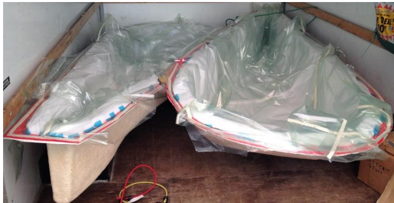
Figure 6: Completed Body Layup
