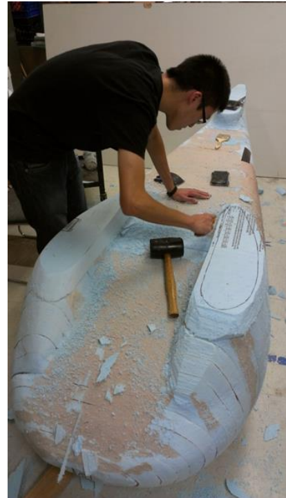
Figure 22: Foam Male Mold Fabrication
