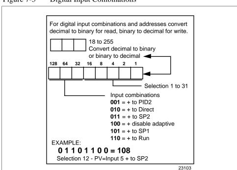
Figure 7-3 Digital Input Combinations
