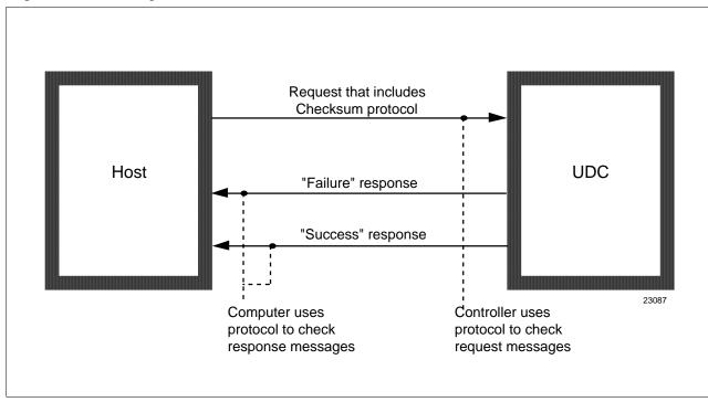
Figure 3-6 Using Checksum Protocol
