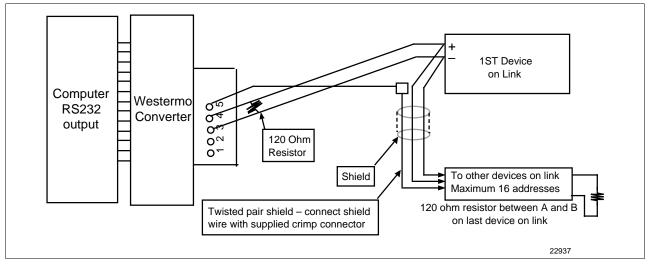
Link devices terminal connections between the Westermo connections and the devices on the communication link.
