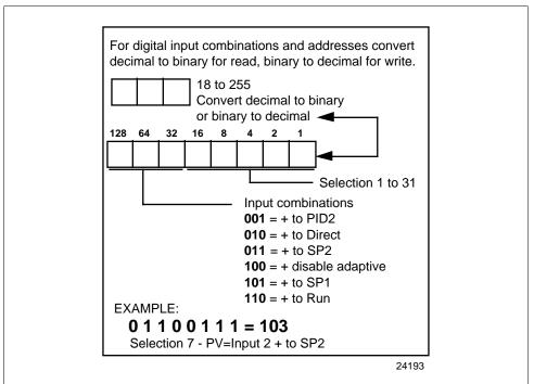
**Communications** Table 9-25 lists all the I.D. codes and ranges or selections for the function parameters in setup group "COM." Loop 1 or 2 is selected in the request message.
