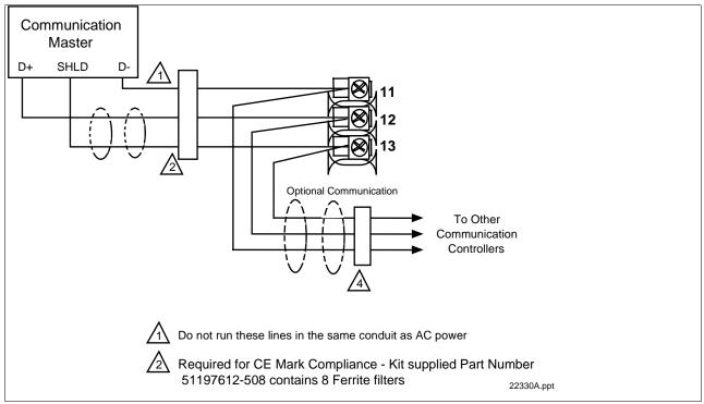
Figure 2-6 UDC5000 Connections (without Digital Input Option)
