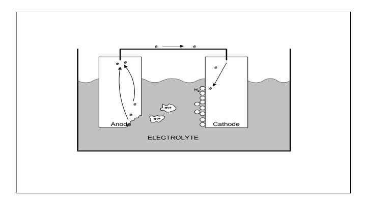
Figure 7 Electrochemical Corrosion Cell
