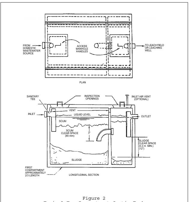
Typical Two-Compartment Septic Tank
