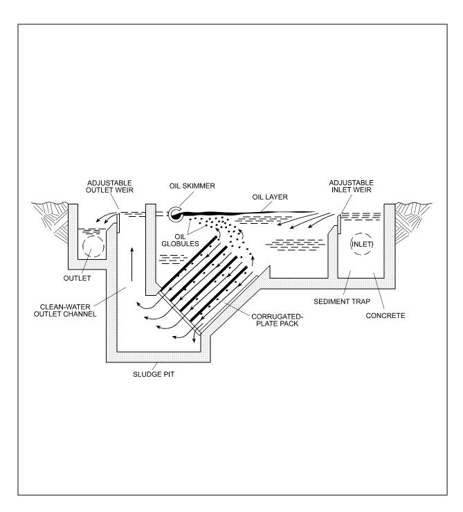
Figure 4 Process Schematic of CPI Separator
