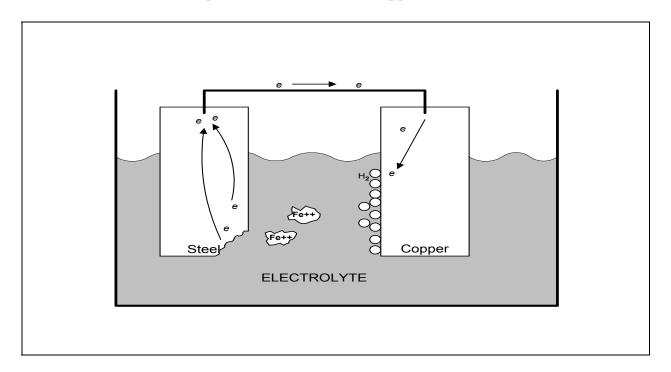
Figure 8 Galvanic Corrosion Cell
