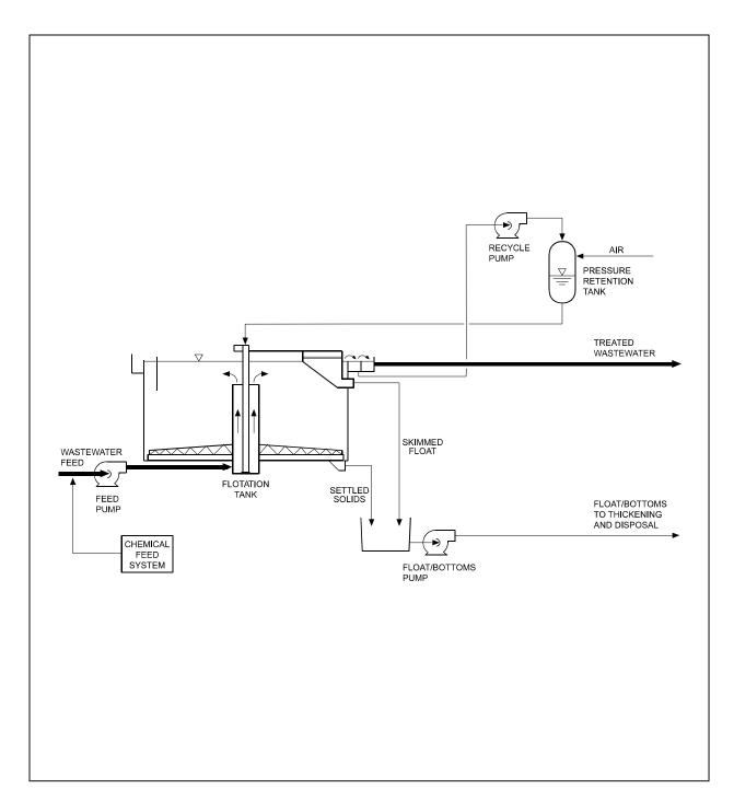
Figure 5 Process Schematic of Dissolved Air Flotation
