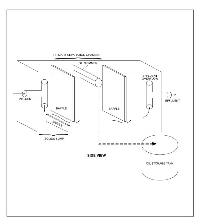
Figure 3 Conventional Gravity Separator
