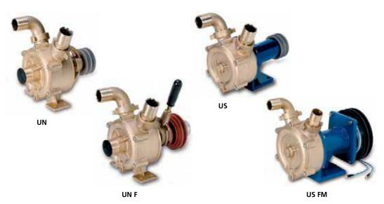
Bidirectional side liquid ring self-priming pumps. Thanks to their high delivery capability, these pumps are widely used in marine applications sector to empty bilges or for sea water suction. Upon request these pumps are also available with BSP thread.
