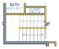
5. While the **Straight Stairs** tool is still active, click in the space to the left of the two stair sections to create a landing.
