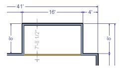
3. Notice that Interior Dimension lines locate the interior side of exterior walls, while other types of dimension lines locate the exterior side.
