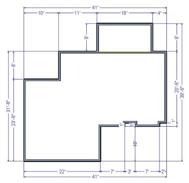
Dimensions can also be used to change the length of a selected wall. Bear in mind, though, that the when a wall is resized in this manner its Start point will always be locked and its End point will always be moved. Because of this, it is often easier to move walls than to resize them. See "Editing Walls" on page 130 of the Reference Manual.
