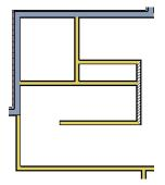
4. Draw a horizontal **Interior Dimension** inside this new room, then use it to move the vertical interior wall 9' 7 3/4" from the opposing exterior wall.
