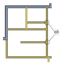
3. Click the **Select Objects** button, then select the top wall section created by the breaks and delete it. Repeat this process for the bottom wall section, so that only the middle section remains, which is hatched in the image below for illustrative purposes.
