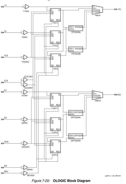
Figure 7-20 illustrates the various logic resources in the OLOGIC block.
