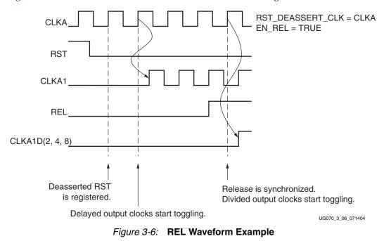
Figure 3-6 illustrates the interaction between the RST and REL signals.
