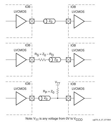
Figure 6-27: LVCMOS Unidirectional Termination
