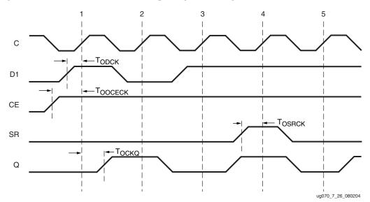
Figure 7-26: OLOGIC Output Register Timing Characteristics
