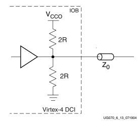
Figure 6-13: Driver with Termination to V<sub>CCO</sub>/2 Using DCI Split Termination
