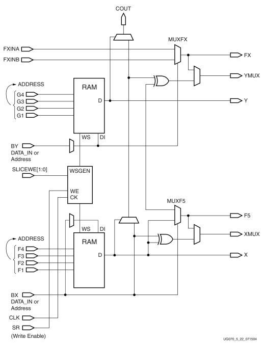
Figure 5-22: Simplified Virtex-4 SLICEM Distributed RAM
