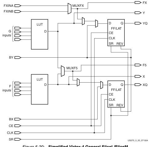
Figure 5-20: Simplified Virtex-4 General SliceL/SliceM
