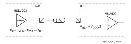
Figure 6-33: HSLVDCI Controlled Impedance Driver with Unidirectional Termination
