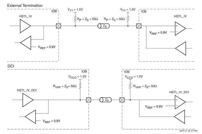
Figure 6-48 shows a sample circuit illustrating a valid bidirectional termination technique for HSTL Class IV.
