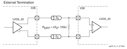
Figure 6-73: LVDS\_25 Receiver Termination
