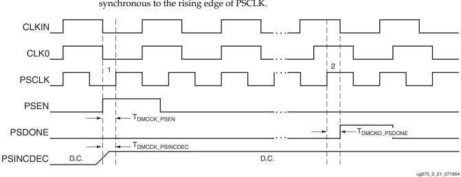
As shown in Figure 2-21, all the variable-phase shift control and status signals are synchronous to the rising edge of PSCLK.
