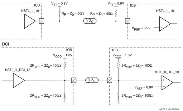
Figure 6-50: HSTL Class II (1.8V) with Unidirectional Termination
