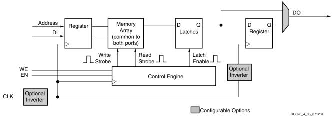
Figure 4-5: Block RAM Logic Diagram (One Port Shown)
