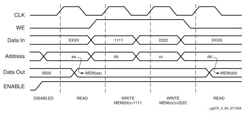
Figure 4-4: NO\_CHANGE Mode Waveforms
