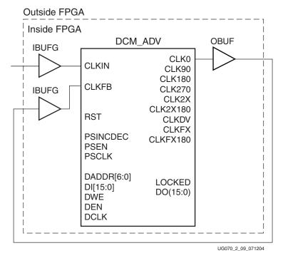
*Figure 2-9:* **Board Level Clock Using OBUF with External Feedback**
