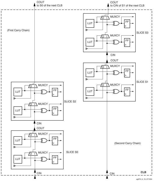
Figure 5-19: Fast Carry Logic Path
