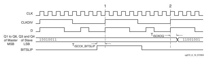
Figure 8-9: Bitslip Timing Diagram
