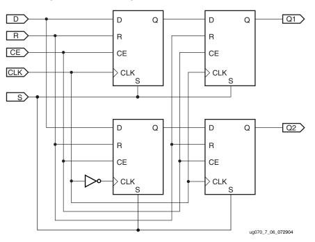
Figure 7-6: Input DDR in SAME\_EDGE\_PIPELINED Mode
