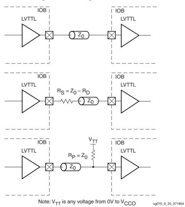
Figure 6-25: LVTTL Unidirectional Termination
