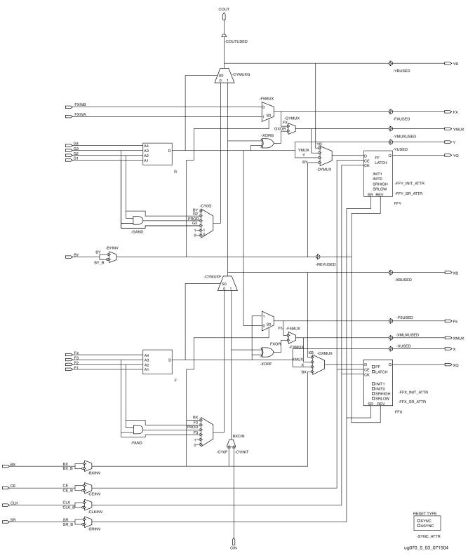
Figure 5-3: Diagram of SLICEL
