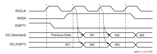
Figure 4-16: Read Cycle Timing (Standard and FWFT Modes)
