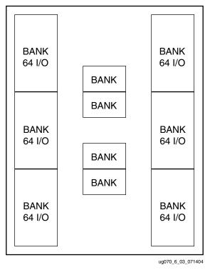
Figure 6-3: Virtex-4 XC4VLX25 I/O Banks
