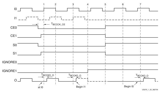
Figure 1-2: BUFGCTRL Timing Diagram
