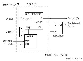
Figure 5-9: Shift Register Configurations
