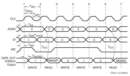
Figure 5-23: Slice Distributed RAM Timing Characteristics
