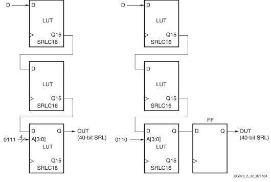
Figure 5-32: 40-bit Static-Length Shift Register
