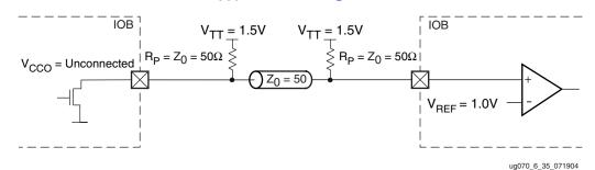
Figure 6-37: GTL+ with External Parallel Termination and Unconnected V<sub>CCO</sub>
