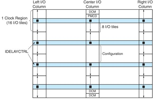
Figure 7-15 illustrates the relative locations of the IDELAYCTRL modules for an XC4VLX15 device.
