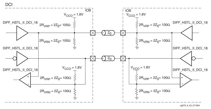
Figure 6-55 shows a sample circuit illustrating a valid termination technique for differential HSTL Class II (1.8V) with bidirectional DCI termination.
