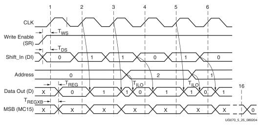
Figure 5-25: Slice SRL Timing Characteristics
