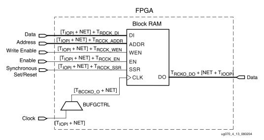
Figure 4-13: Block RAM Timing Model
