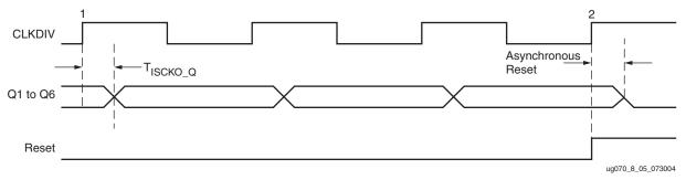
Figure 8-5: ISERDES Output Data Timing Diagram
