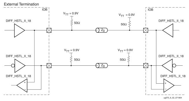
Figure 6-54: Differential HSTL (1.8V) Class II Bidirectional Termination
