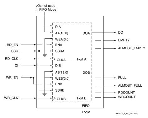
I/Os used for the FIFO implementation. The "Built-in FIFO Support" section contains further details.
