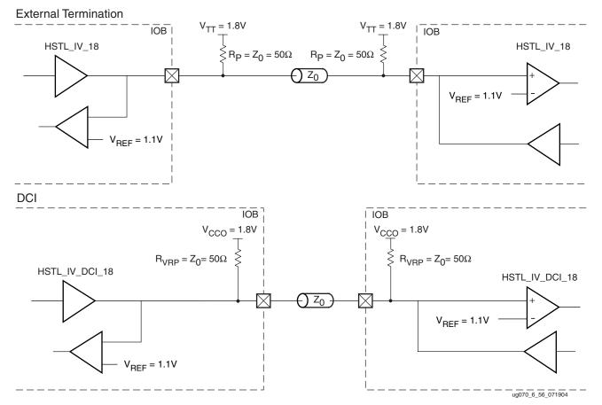
Figure 6-58: HSTL Class IV (1.8V) with Bidirectional Termination
