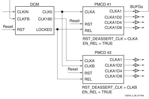
Figure 3-8: DCM and Parallel PMCDs
