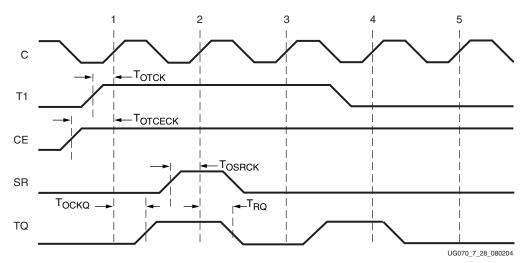
Figure 7-28: OLOGIC 3-State Register Timing Characteristics
