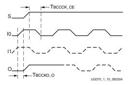
Figure 1-10: BUFGMUX\_1 Timing Diagram
