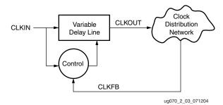
Figure 2-3: Simplified DLL Circuit
