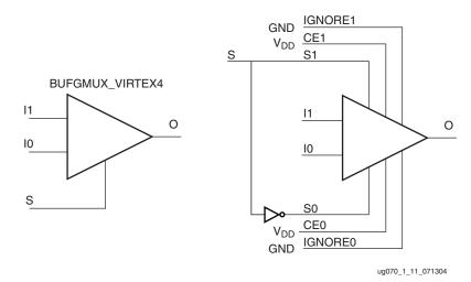
*Figure 1-11:* **BUFGMUX\_VIRTEX4 as BUFGCTRL**
