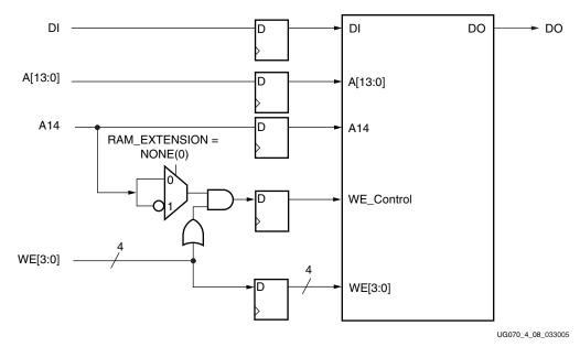
Figure 4-8: Byte-Wide Write Enable In Block RAM
