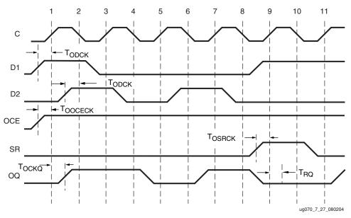
Figure 7-27 illustrates the OLOGIC ODDR register timing.
