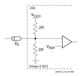
Figure 6-9: Input Termination to V<sub>CCO</sub>/2 Using DCI Split Termination
