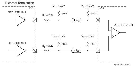
Figure 6-69: Differential SSTL (1.8V) Class II Unidirectional Termination
