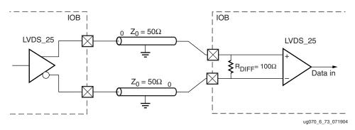
Figure 6-75: LVDS\_25 With DIFF\_TERM Receiver Termination
