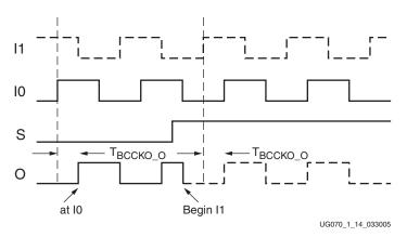
*Figure 1-14:* Asynchronous Mux Timing Diagram
