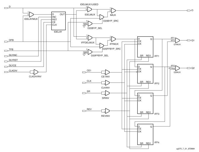
Most of the control signals have an optional inverter. Any inverter placed on a control signal is automatically absorbed into the ILOGIC block (i.e., no CLBs are used).
