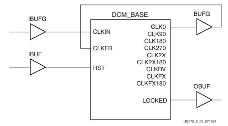
The circuit in Figure 2-7 shows DCM\_BASE implemented with internal feedback and access to RST and LOCKED pins. This example shows the simplest use case for a DCM.
