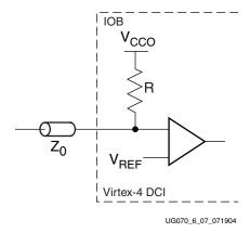
Figure 6-7: Input Termination Using DCI Single Termination
