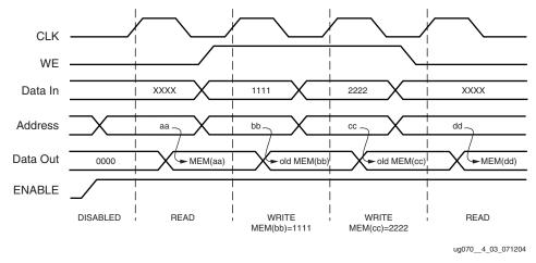
Figure 4-3: **READ\_FIRST Mode Waveforms**
