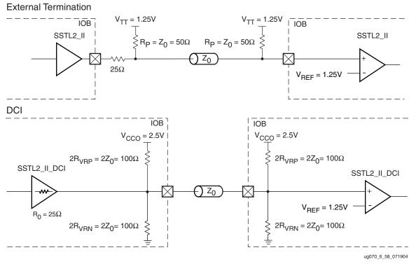
Figure 6-60: SSTL2 Class II with Unidirectional Termination
