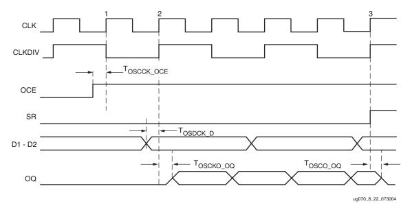
Figure 8-13: OSERDES 2:1 SDR Data Serialization Timing Diagram
