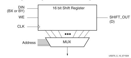
Figure 5-10 is an equivalent representation of the shift register.
