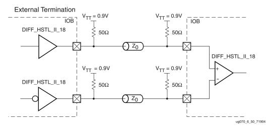
Figure 6-52: Differential HSTL (1.8V) Class II Unidirectional Termination
