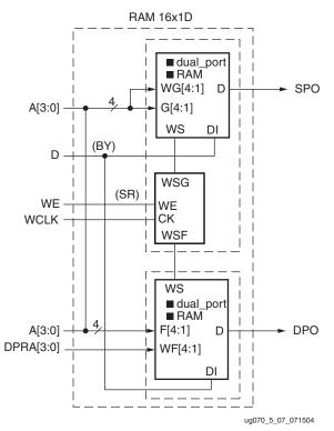
Figure 5-7: Dual-Port Distributed RAM (RAM16x1D)
