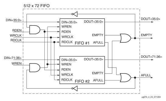
Figure 4-23: Cascading FIFO by Width
