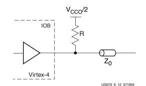
Figure 6-12: Driver with Termination to V<sub>CCO</sub>/2 without DCI
