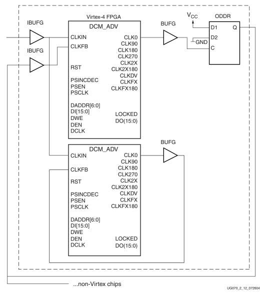
The example in Figure 2-12 shows an interface from Virtex-4 FPGAs to non-Virtex devices.
