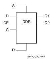
Figure 7-8: IDDR Primitive Block Diagram
