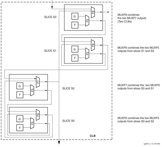
Figure 5-13: MUXF5 and MUXFX Multiplexers
