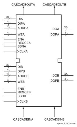
Figure 4-9 illustrates all the I/O ports of the block RAM primitive (RAMB16).
