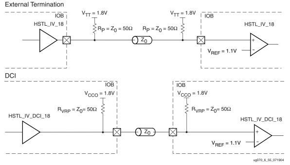
Figure 6-57: HSTL Class IV (1.8V) with Unidirectional Termination
