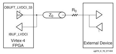
Figure 6-80: 3.3V I/O Configuration
