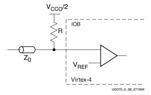
Figure 6-8: Input Termination to V<sub>CCO</sub>/2 without DCI
