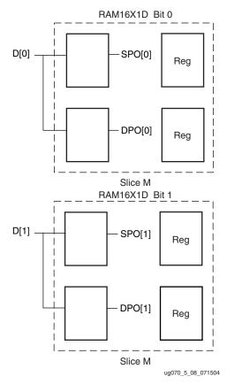
*Figure 5-8:* **Two RAM16X1D Placement**
