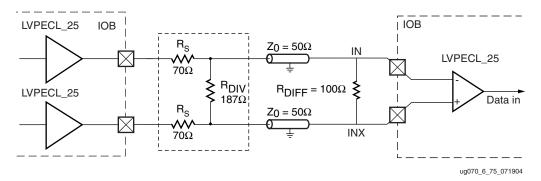
Figure 6-77: LVPECL Transmitter Termination
