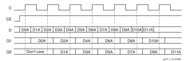
Figure 7-5: Input DDR Timing in SAME\_EDGE Mode
