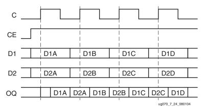
Figure 7-24: Output DDR Timing in SAME\_EDGE Mode
