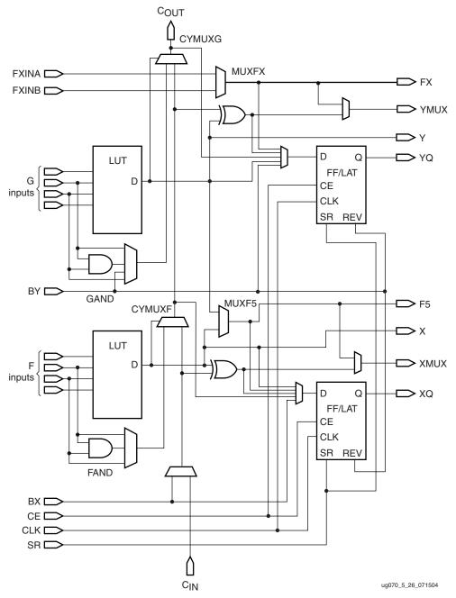
Figure 5-26: Simplified Virtex-4 Slice Carry-Chain Diagram
