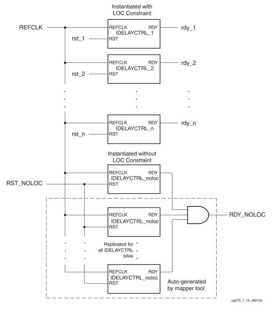
The circuitry that results from instantiating the IDELAYCTRL components as shown is illustrated in Figure 7-19.
