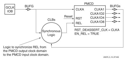
Figure 3-10: PMCD Driven by BUFG and Synchronous Logic
