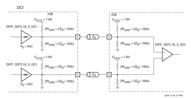
Figure 6-70 shows a sample circuit illustrating a valid termination technique for CSE differential SSTL Class II (1.8V) with unidirectional DCI termination.
