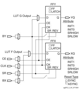
Figure 5-4: Register/Latch Configuration in a Slice
