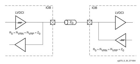
Figure 6-30: Controlled Impedance Driver with Bidirectional Termination
