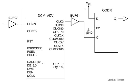
Figure 2-10: Board Level Clock with Internal Feedback
