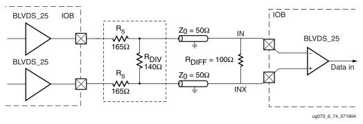
Figure 6-76: BLVDS Transmitter Termination
