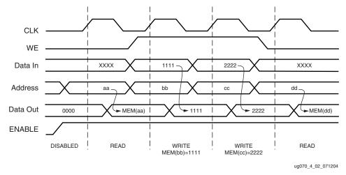
Figure 4-2: WRITE\_FIRST Mode Waveforms
