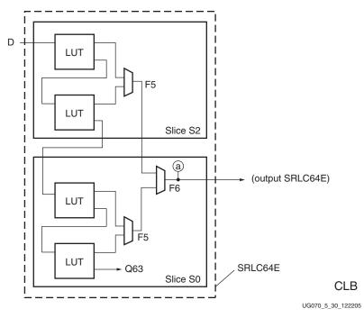
Figure 5-30: Shift Register Placement
