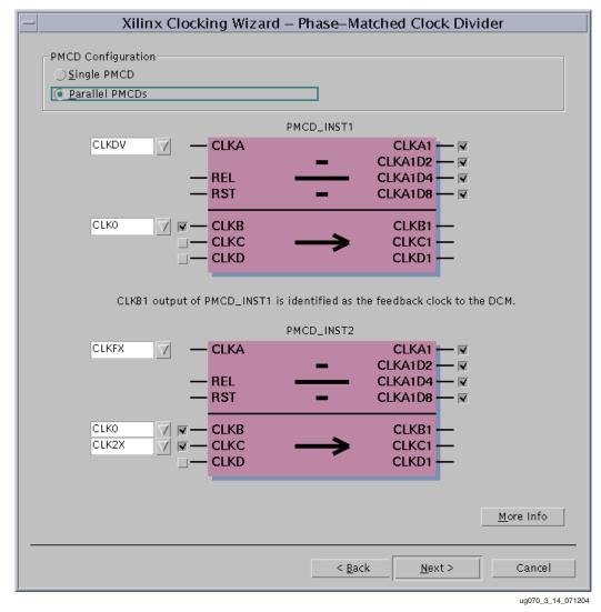
Figure 3-14: Xilinx Clocking Wizard - Phase-Matched Clock Divider (PMCD)
