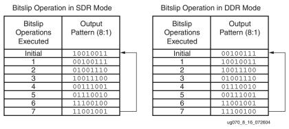
Figure 8-7: Bitslip Operation Examples
