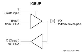
Figure 6-20: Input/Output Buffer (IOBUF) Primitive
