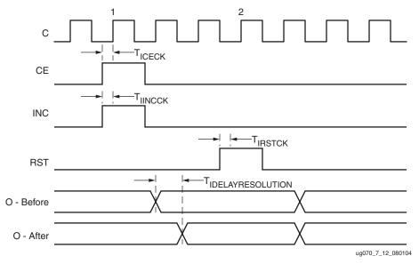
Figure 7-12: IDELAY Timing Diagram
