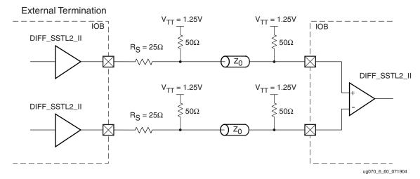
*Figure 6-62:* Differential SSTL2 Class II Unidirectional Termination
