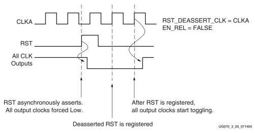
Figure 3-5 illustrates an RST waveform when EN\_REL = FALSE.
