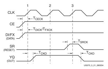
Figure 5-21: General Slice Timing Characteristics
