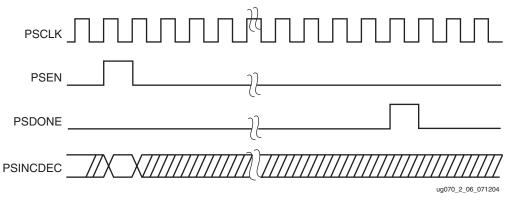
Figure 2-6: Phase-Shift Timing Diagram
