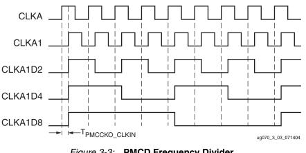
Figure 3-3: PMCD Frequency Divider
