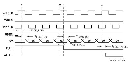
Figure 4-19: Reading From a Full FIFO
