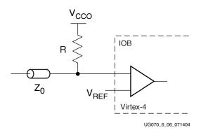
Figure 6-6: Input Termination to V<sub>CCO</sub> without DCI
