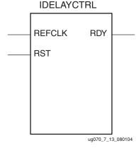
Figure 7-13: IDELAYCTRL Primitive
