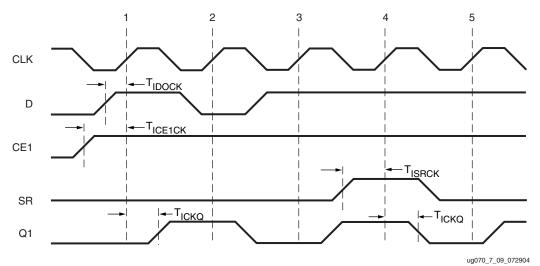
Figure 7-9: ILOGIC Input Register Timing Characteristics
