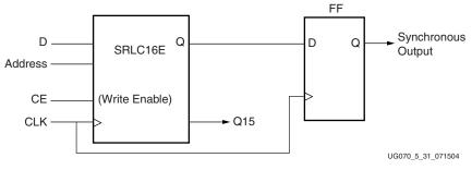
Figure 5-31: Fully Synchronous Shift Register
