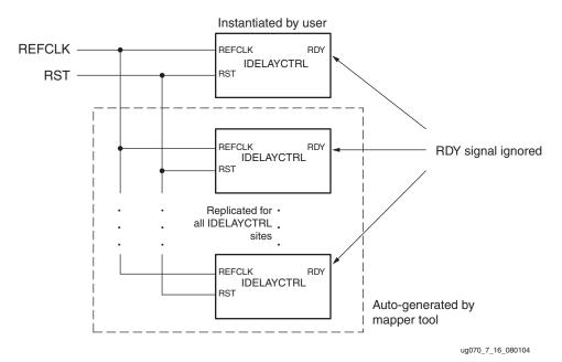
Figure 7-16: Instantiate IDELAYCTRL Without LOC Constraints - RDY Unconnected
