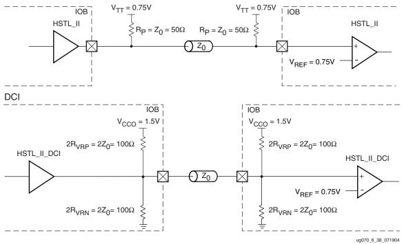
Figure 6-40: HSTL (1.5V) Class II Unidirectional Termination
