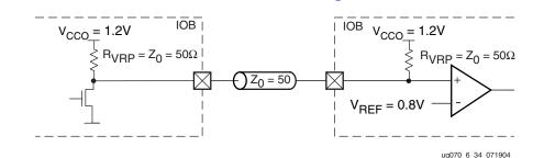
A sample circuit illustrating a valid termination technique for GTL\_DCI with internal parallel driver and receiver termination is shown in Figure 6-36.
