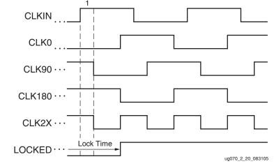
Figure 2-20: Phase Shift Example: Fixed
