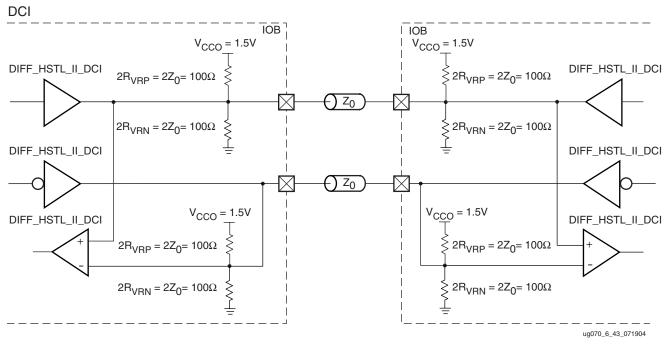
Figure 6-45: Differential HSTL (1.5V) Class II DCI Bidirectional Termination
