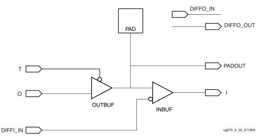
Figure 6-2: Basic IOB Diagram
