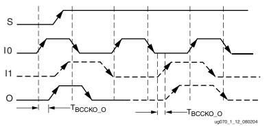
*Figure 1-12:* **BUFGMUX\_VIRTEX4 Timing Diagram**
