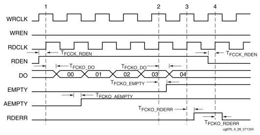
Figure 4-20: Reading From an Empty / Almost Empty FIFO (Standard Mode)
