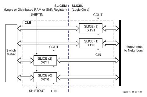
Figure 5-1: Arrangement of Slices within the CLB
