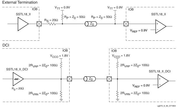
Figure 6-67: SSTL18 (1.8V) Class II Unidirectional Termination
