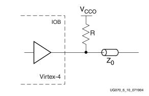
Figure 6-10: Driver with Termination to V<sub>CCO</sub> without DCI
