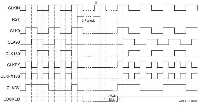
Figure 2-19: RESET/LOCK Example
