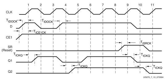
Figure 7-10: ILOGIC in IDDR Mode Timing Characteristics
