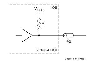
Figure 6-11: Driver with Termination to V<sub>CCO</sub> Using DCI Single Termination
