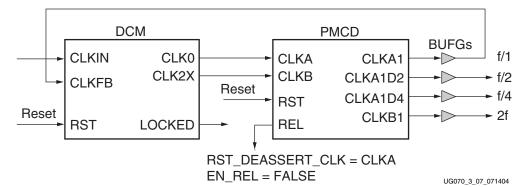
Figure 3-7: DCM and a Single PMCD
