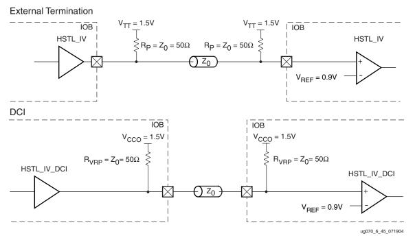
Figure 6-47: HSTL Class IV Unidirectional Termination
