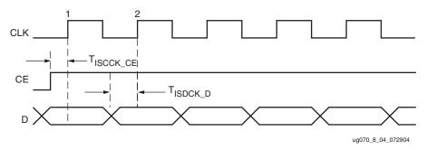
Figure 8-4: ISERDES Input Data Timing Diagram
