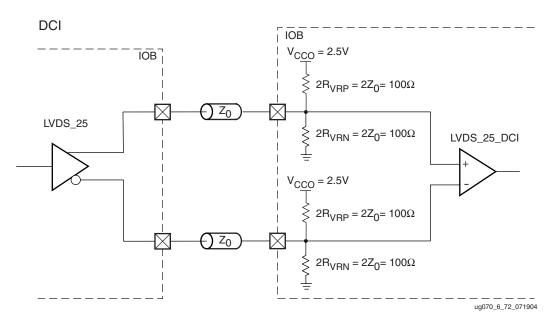
Figure 6-74: LVDS\_25\_DCI Receiver Termination
