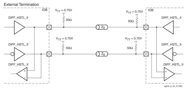
Figure 6-44: Differential HSTL (1.5V) Class II Bidirectional Termination
