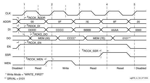
Figure 4-12: Block RAM Timing Diagram
