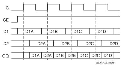
Figure 7-22: Output DDR Timing in OPPOSITE\_EDGE Mode
