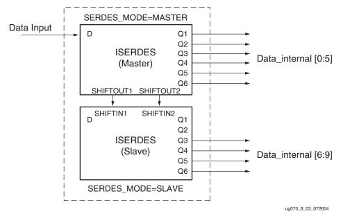
*Figure 8-3:* Block Diagram of ISERDES Width Expansion
