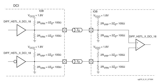
Figure 6-53 shows a sample circuit illustrating a valid termination technique for differential HSTL Class II (1.8V) with unidirectional DCI termination.
