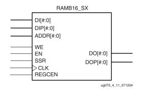
Figure 4-11: Single-Port Block RAM Primitive
