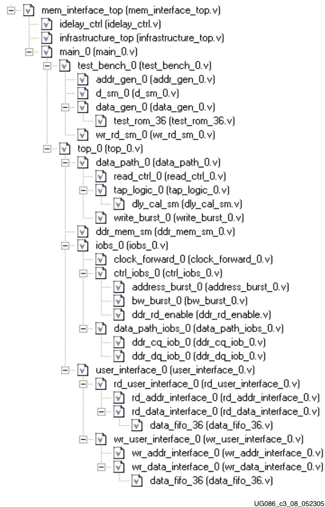
Figure 5-3: DDRII SRAM Controller Hierarchy
