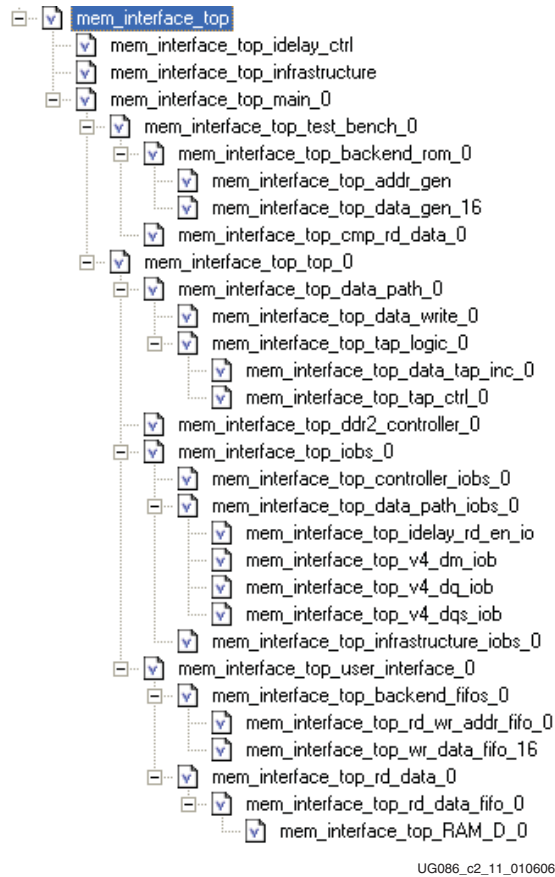
Figure 3-10: Hierarchical Structure of the DDR2 SDRAM Design (SerDes Clocking)
