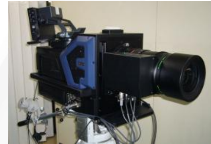
Full-resolution camera (2010) 33 M pixel x 3-sensor, 65 kg
