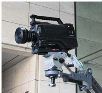
Portable camera 33 M pixel x 1-sensor 5 kg
