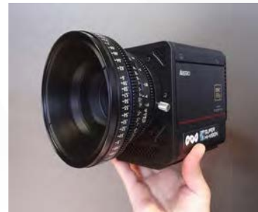
Cube camera 33 M pixel x 1-sensor 2 kg
