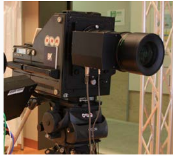
120 Hz 3-chip full-spec. camera 33 M pixel × 3-sensor, 60 kg
