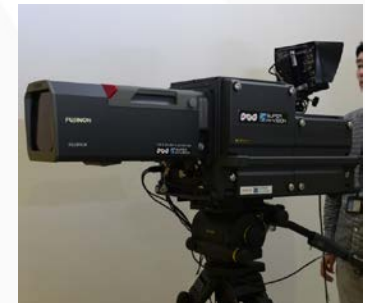
High sensitive theatre camera 33 M pixel x 3-sensor 48 kg
