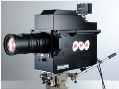
1st generation camera (2002) 8 M pixel x 4-sensor, 80 kg
