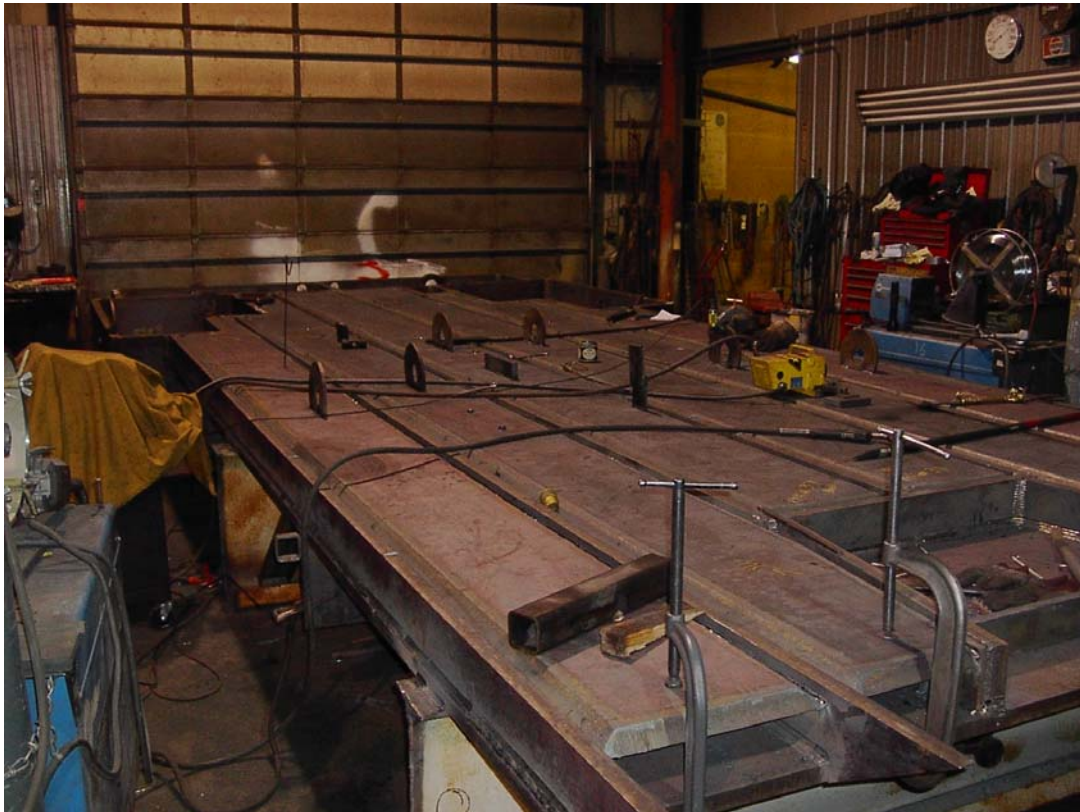
Miner trailer in work, showing the reinforcement on the bottom
