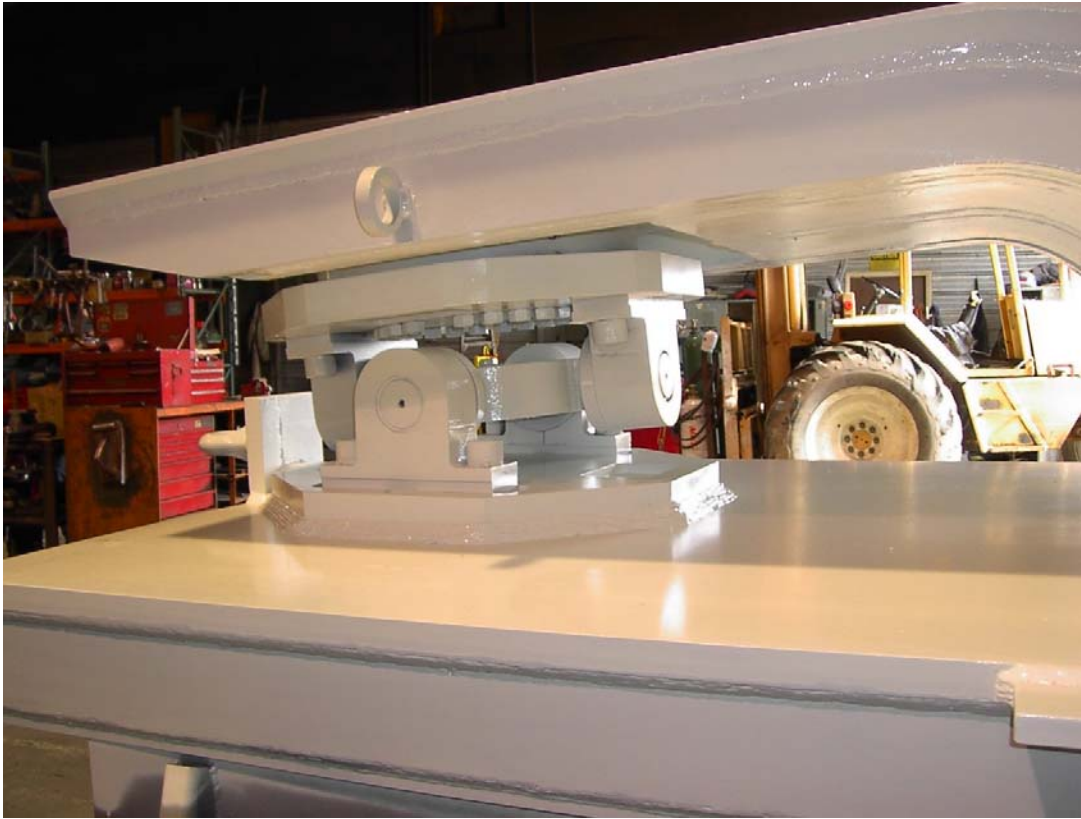
Cookiesheet to gooseneck attachment
