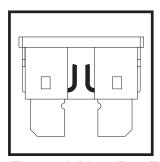
Figure 21A. Blown Fuse (Replace)
