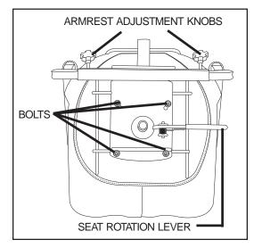
Figure 11. Seat Adjustments
