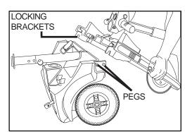
Figure 20. Frame Separation
