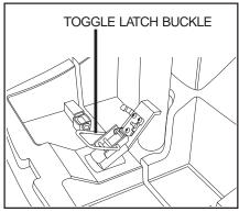
Figure 18A. Toggle Latch (Unlatched)
