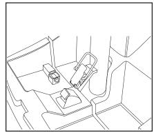
Figure 18B. Toggle Latch (Secured For Disassembly)
