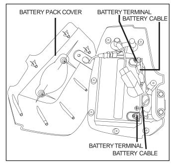
Figure 9. Battery Replacement
