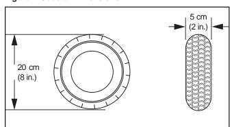
Figure 4A. Front Tyre Dimensions
