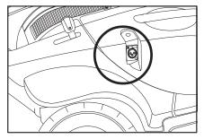
Figure 8. Charger Power Lead Receptacle
