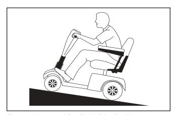
Figure 2A. Increased Stability Driving Position
