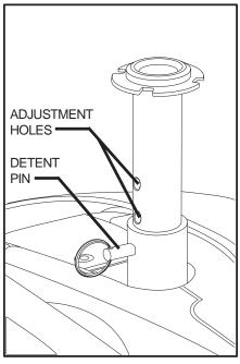
Figure 12. Seat Height Adjustment
