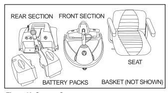
Figure 13. Scooter Components
