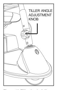
Figure 10. Tiller Angle Adjustment Knob
