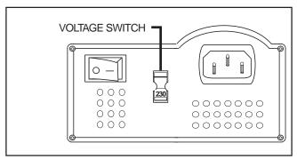
Figure 7A. Voltage Switch
