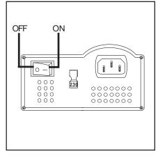
Figure 8A. Charger On/Off Switch
