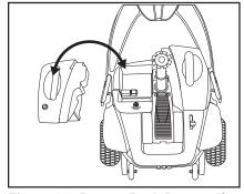
Figure 16. Battery Pack Removal/Installation
