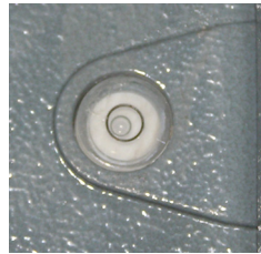
Figure 2.2 Adjust feet until bubble is centered in black circle
