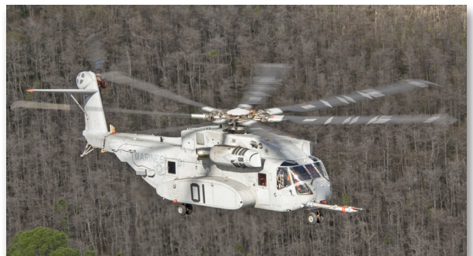
The CH-53K Heavy Lift Replacement helicopter was designed to carry about three times the load of the CH-53E yet fit the same deck footprint. (US Navy)
