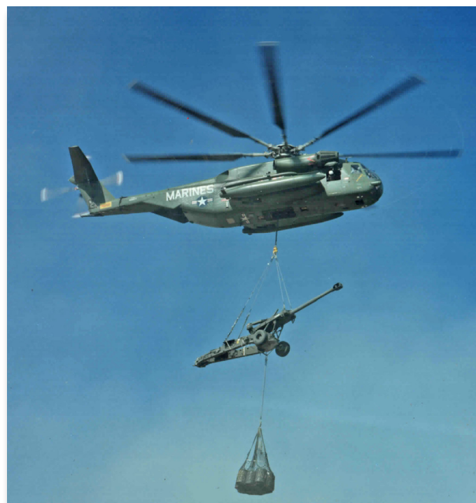
The CH-53D with -413 engines upped the Sea Stallion gross weight to 42,000 lb. (Sikorsky Archives)
