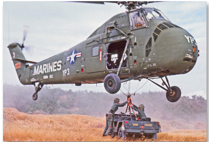
The S-58 or HUS-1 was the Marine medium lift helicopter early in the Vietnam war. (Sikorsky Archives)
