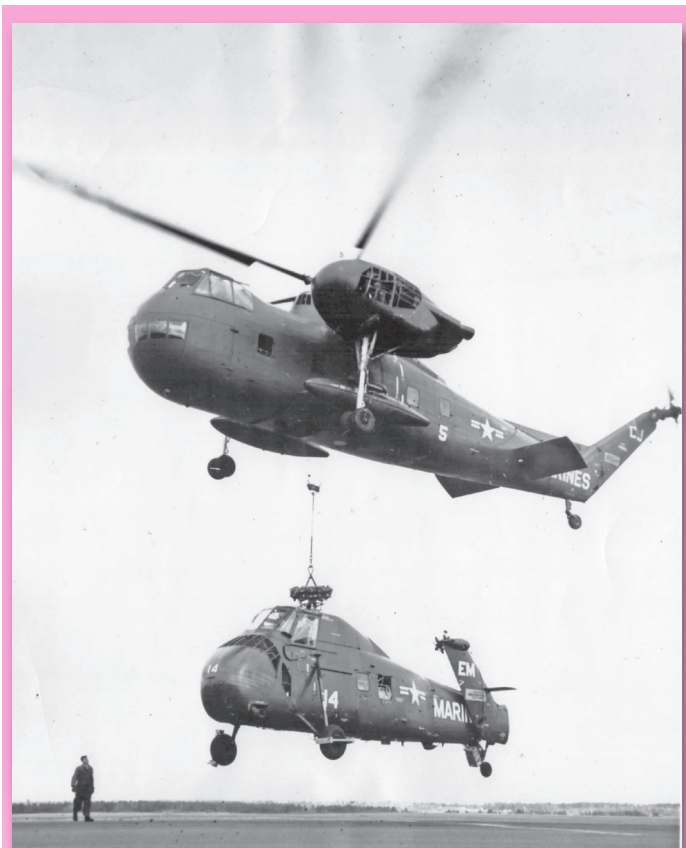
The HR2S-1 lifts a Sikorsky HUS (S-58) in a downed aircraft recovery exercise. (Sikorsky Archives)
