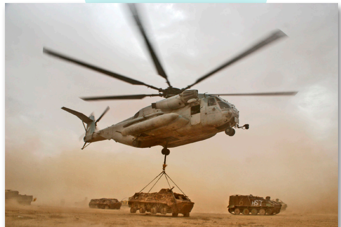
The CH-53E used the power of three T64 engines and seven main rotor blades to haul heavy cargo for the Marines. (Sikorsky Archives)
