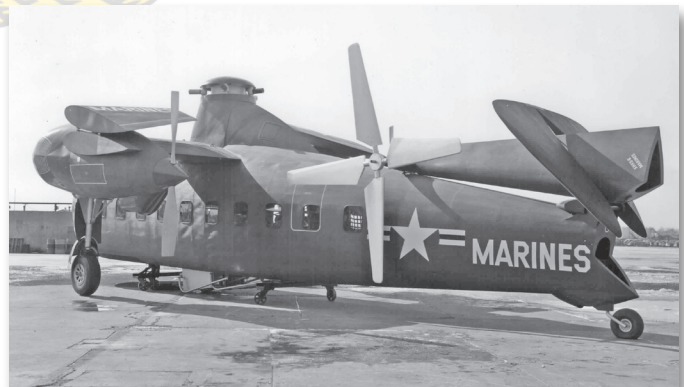
Sikorsky mocked up the S-56B with pusher turboprops and folding wings. (Sikorsky Archives)
