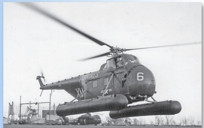
Marine Helicopter Squadron HMX-1 was the test unit for helicopter development. Here, an S-55 or Marine HRS flies with floats for water landings. (Sikorsky Archives)
