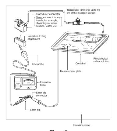
**<u>Figure 3</u>** Recommended TEE Transducer Test Setup for Toshiba TEE Transducers Using the Toshiba Tester (Hioki Model 3451 Digital Megohm Insulation HiTester)<sup>3</sup>
