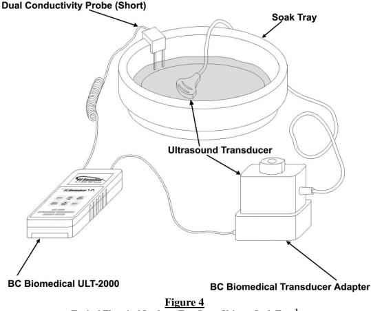
Typical Electrical Leakage Test Setup Using a Soak Tray<sup>3</sup>
