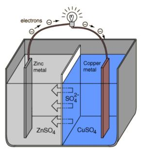
**Example of a Simple Voltaic Cell**
