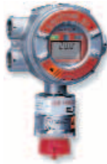
Electrochemical Sensors for monitoring various toxics and oxygen
