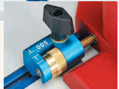
▲ Fine Tuning. This micro-adjuster makes it easy to precisely tweak the fence setting.
