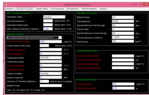
Figure 6: Operational properties of subsea pipeline.
