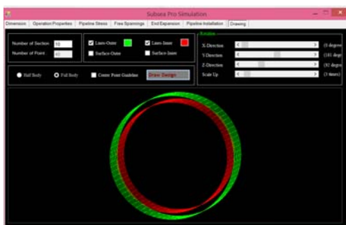
Figure 9: Design of selected wall thickness at ultra-deep water using Subsea Pro Simulation software
