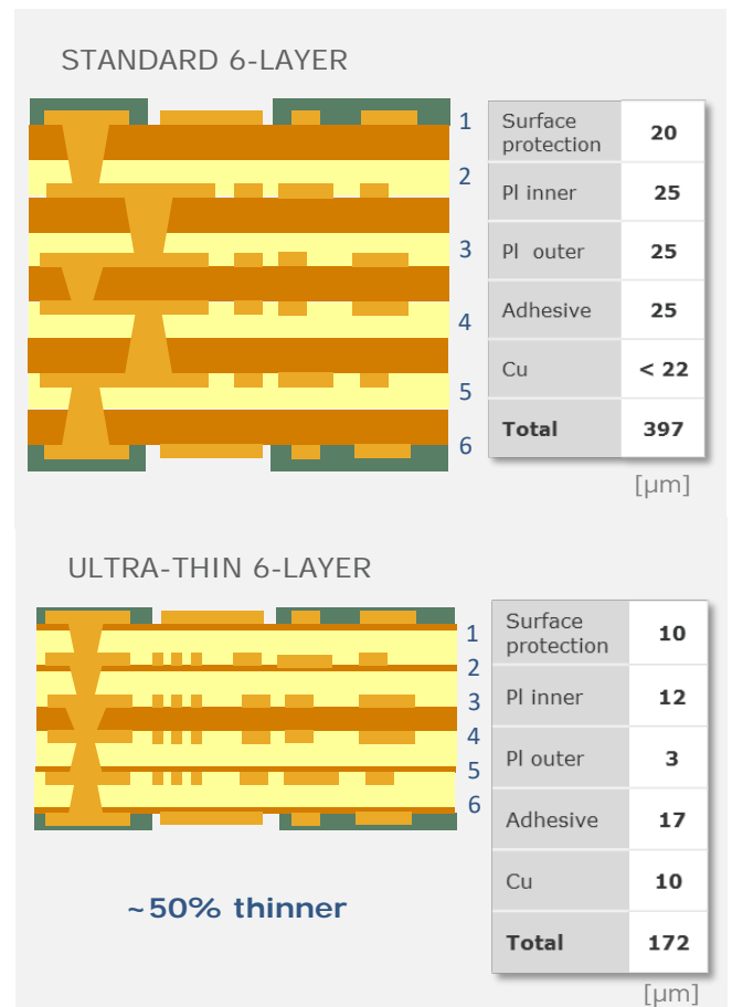
Figure 2. 6-layer stack-up with standard flex material compared to 6-layer stack-up with ultra-thin base material
