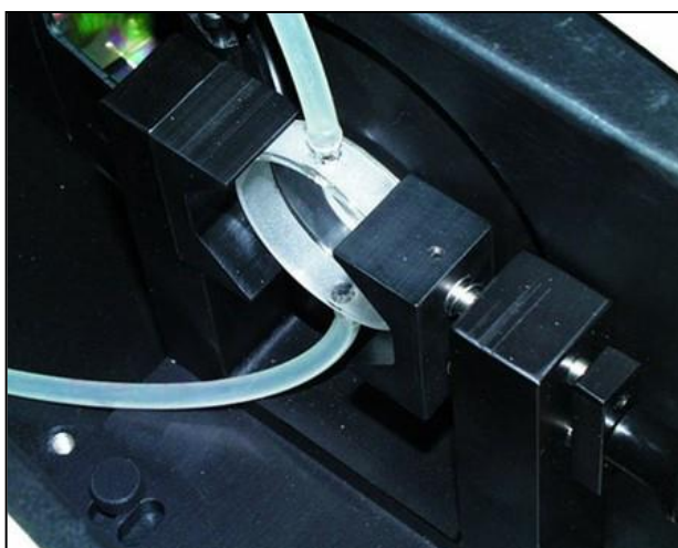
Figure 57. Flow Cell Installed
