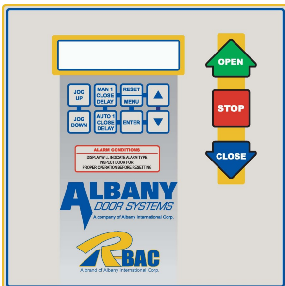
Figure 1 Control Panel Key
