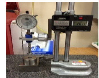
Measuring hole diameter
