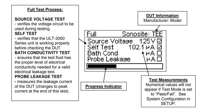
**BATH TEST SCREEN** – This screen is accessed from the Main Screen by pressing the
