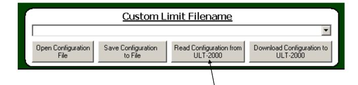
In the "Custom Limit Filename" window, click "Read Configuration from ULT-2000" to view the custom transducer configuration currently stored on the device. The loaded Manufacturers and Models are displayed in the respective labeled windows. The user may alter these transducer settings if desired.
