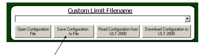
Using the "Save Configuration to File" button in the "Custom Limit Filename" window, the user may save the manipulated Custom Limit Configuration. This allows the user to download the changes at a later time, or to download the changes to several ULT-2000 series devices. Clicking "Save Configuration to File" prompts a save window which allows the user to name the Custom Limit Configuration. Below is a sample save window.
