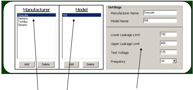
Select the Manufacturer and Model to be altered. Within the "Settings" window, enter the desired changes including Manufacturer Name, Model Name, Lower and Upper Leakage Limits, Test Voltage, and Frequency. To submit the changes to the ULT-2000 series, click "Download Configuration to ULT-2000" in the "Custom Limit Filename" window.
