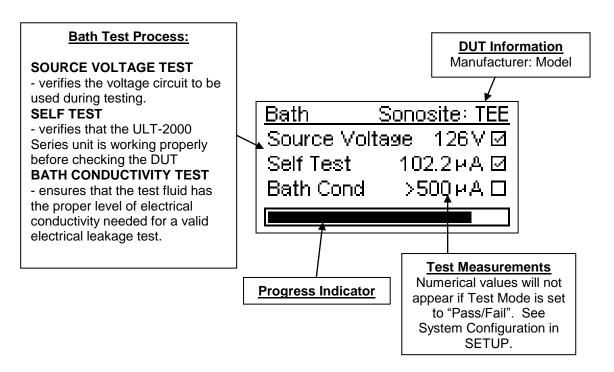
**TEST MESSAGES** – Messages appear after each FULL or BATH test is completed.
