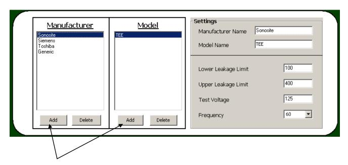
Using the "Add" buttons in the "Manufacturer" and "Model" windows, the user may create a Manufacturer and/or Model entry. If the desired Manufacturer is not currently displayed, click "Add" in the Manufacturer window. This introduces two "New" entries, one each in the "Manufacturer" and "Model" windows. See the previous section to alter the "New" transducer settings.
