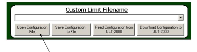
Using the "Open Configuration File" button in the "Custom Limit Filename" window, the user may open saved Custom Limit Configurations. This allows the user to download the saved Custom Limit Configuration to several ULT-2000 series devices. Clicking "Open Configuration File" prompts a load window which allows the user to select the desired Custom Limit Configuration. Below is a sample load window.
