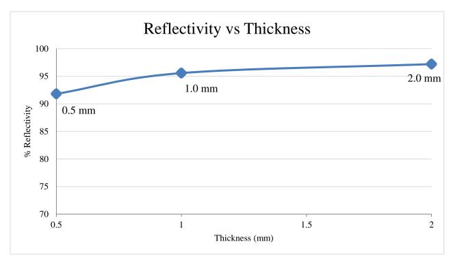
Figure 4: Reflectivity vs Thickness of Samples with the Same Porosity
