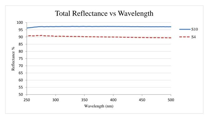
**Figure 2:** Total Reflectance. Sample 4 (Porous PTFE sheet at 0.5mm thickness) and Sample 10 (2 mm thick porous PTFE sheet) bracket the low and high UV reflectivity of the PTFE samples in the experimental set.
