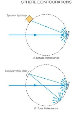
Figure 1: Reflectivity Test Setup.
