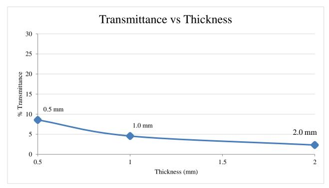
Figure 5: Transmittance as a function of Thickness of Samples with the Same Porosity
