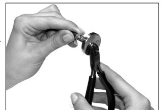
Fig. 28: Shortening of the out standing bare fibre
