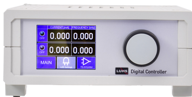
Fig. 19: DC-0030 Dual channel LED transmitter
