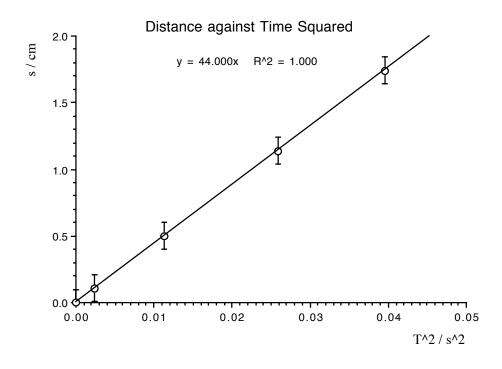
Acceleration:  $a = 2 \times slope = 2 \times (44.0 \text{ cm s}^{-2}) = 88.0 \text{ cm s}^{-2} \approx 88 \text{ cm s}^{-2}$
