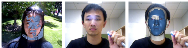
Figure 14: Limitations of our system. Left: since our RGB-D camera is based on IR illumination, our depth map can be negatively affected by direct sunlight. Middle/Left: Illuminating the directly face with a flashlight produces an outlier during face segmentation.
