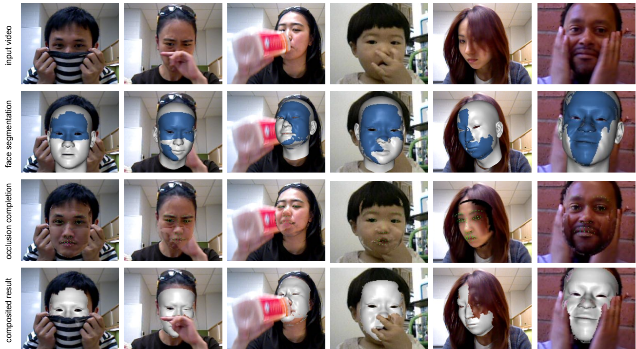
Figure 8: Our facial tracking results. We can handle challenging cases with large occlusion such as those caused by wearable accessories, hand-to-face gestures, hair and other obstacles. From top to bottom, we show the frames of input video, tracking models with inliers visualized in blue, synthesized face textures with 2D facial features, and the final composited results.
