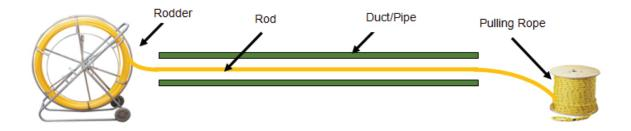
Figure 1 Pulling rope installation by rodder
