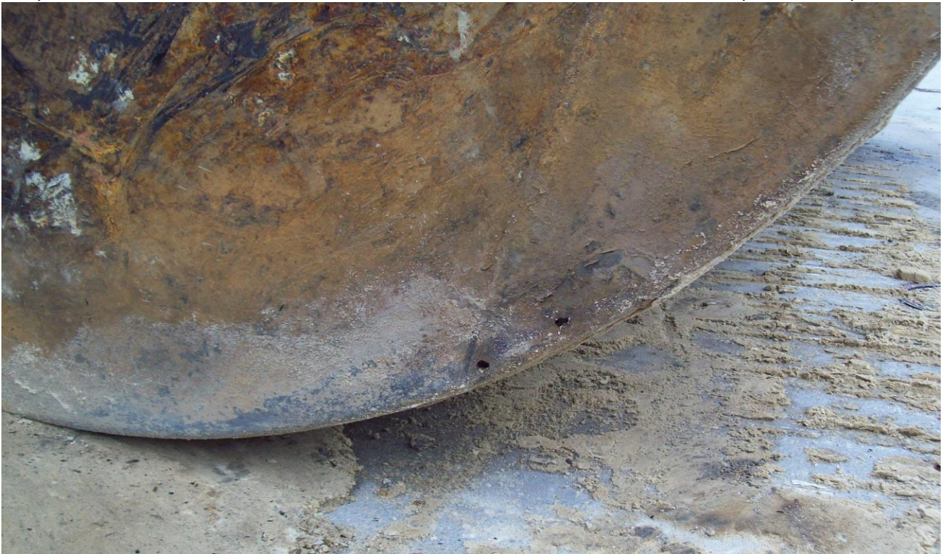
Bottom photo: a documented release. This is the same tank as above. Note the two quarter-size perforations.
