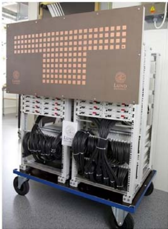
Lund-NI massive MIMO prototype 128 elements, 30.72 Mbps in 20 MHz
