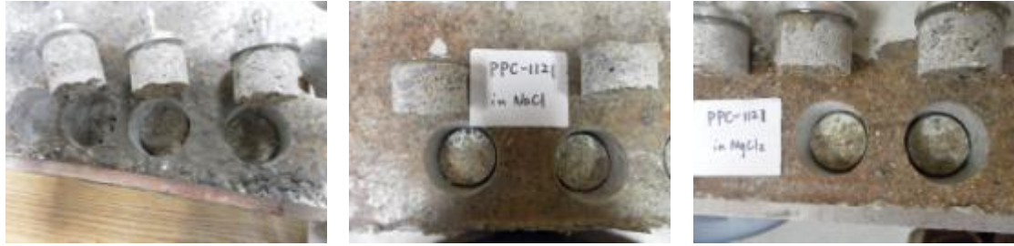
Figure 7.9: Digital photos of concrete samples after bond strength tests
