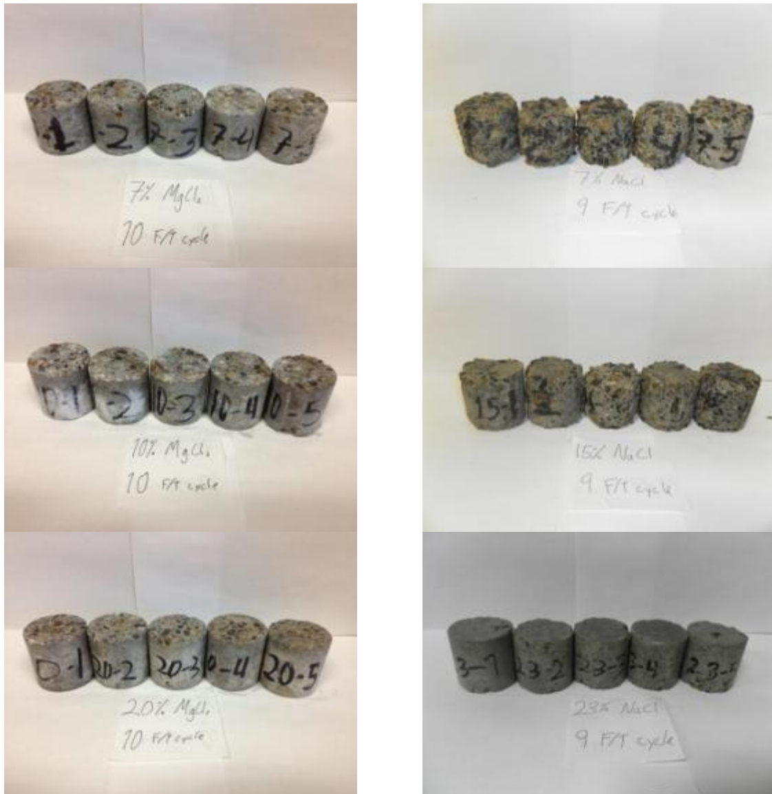
Figure 3.14: Lab concrete samples exposed to 10 F/T cycles in MgCl_2 and NaCl solutions, respectively
