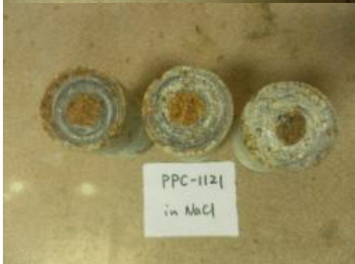
Figure 7.13: Abrasion test surfaces of cored overlay cylinders after freeze/thaw and wet/dry cycles in 15% NaCl solutions
