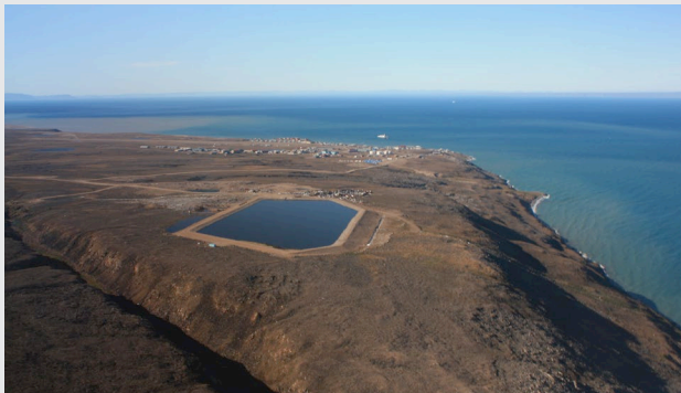
Figure 1. Overhead photograph of the single cell WSP in Pond Inlet, Nunavut.
