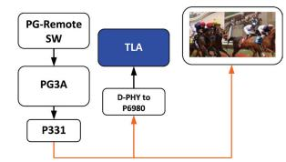
Figure 20. Typical Setup for Display Testing.
