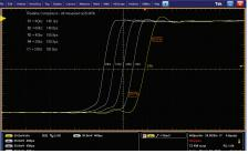
Figure 6. Risetime measurements at various bandwidths.
