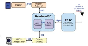
Figure 1. Block diagram of a typical mobile device.
