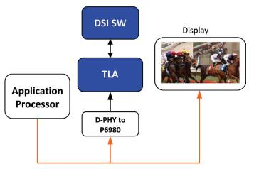
Figure 15. Typical Setup for DSI Digital Debug.
