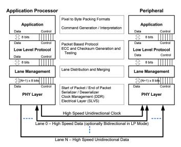
Figure 12. MIPI DSI Layered Architecture.
