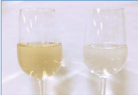
Figure 5a: Color correction of white wine with SUPRAdisc™ AKS sheet-based modules – before ( left ) and after ( right ) treatment
