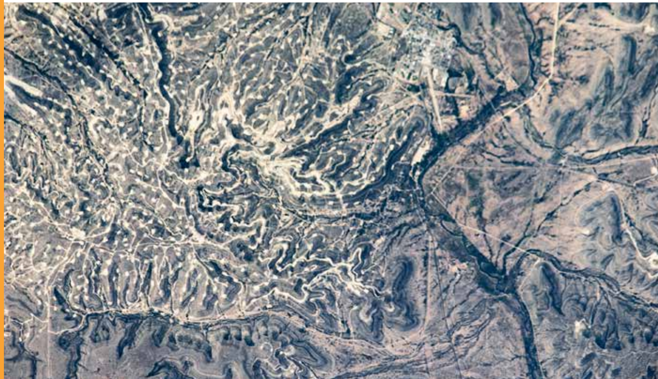
WHITE WELL LOCATIONS AND PETROLEUM DRILLING STRUCTURES MARK THE YATES OIL FIELD IN THE LAYERED SEDIMENTARY ROCKS OF THE PERMIAN BASIN. ACTIVITIES RELATED TO OIL AND GAS PRODUCTION IN THIS AREA OF WEST TEXAS MAY HAVE CONTRIBUTED TO THREE THOUSAND EARTHQUAKES DETECTED NEAR PECOS THROUGHOUT 2018. CREDIT: EARTH SCIENCE AND REMOTE SENSING UNIT, NASA JOHNSON SPACE CENTER
