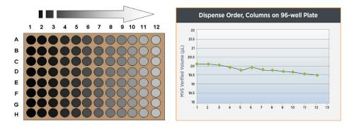
A schematic representation of a 96-well microtiter plate showing volume dispense trending. In this representation, an 8-channel device was used to dispense 20 µL across the plate from column 1 to column 12 (left). Although the volumes in each column should be identical, the actual volume is sequentially lowering (drifting downward) with each dispense (right).
