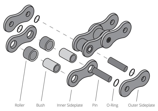
You probably know by now that chains need proper lubrication at regular intervals to function properly and to prevent wear. If you have a chain driven bike you know that sometimes chain adjustments have to be made, pushing the rear wheel further back to take up the slack of the chain. So how do chains actually wear?
