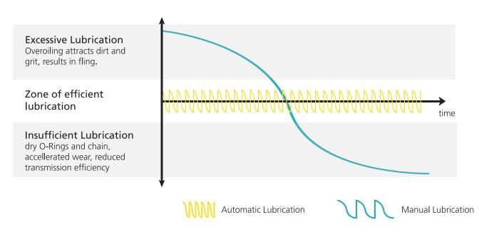
In a recent customer survey Scottoiler users reported, on average, a 2.98 times longer chain life with their automatic chain oiler. With the cost for a basic set of chain and sprockets exceeding more than £100/\$150, not including workshop time, a Scottoiler will have paid for itself after your first set of chain and sprockets.
