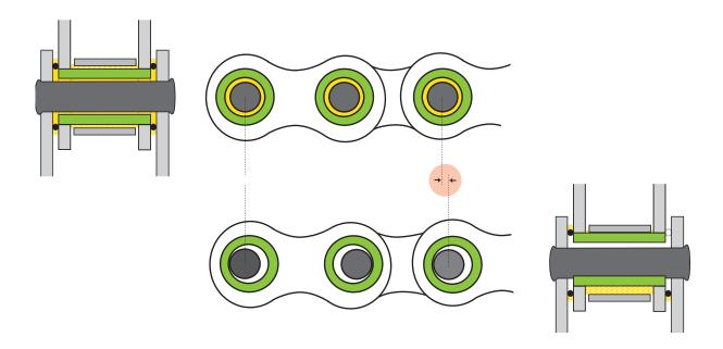
However a chain is only as strong as its weakest link and will also fail quickly if just one chain link is subject to excessive wear, possibly due to a quality error or lack of lubrication. Your chain and sprockets rely on a delicate interplay to transfer power efficiently.
