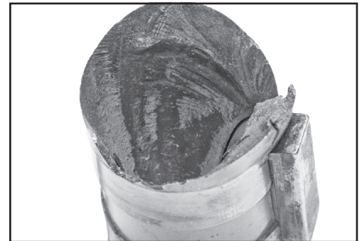
Shaft failure due to cyclic loading
