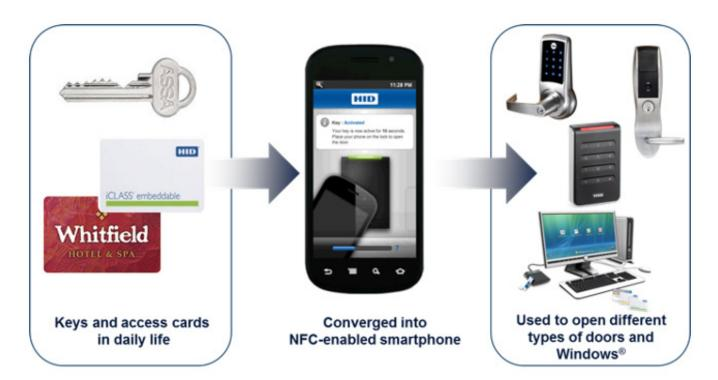
Especially for Access Control - also Bluetooth Low Energy (BLE) may be used as alternative technology to NFC. As an advantage it works with all modern phones, but requires BLE enabled door locks whereas NFC can interact with existing infrastructure. See for example the <u>Starwood Preferred Guest keyless entry service</u>.
