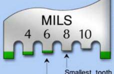
After the gauge is removed from the substrate, observe the MIL value of the largest tooth or notch that is wet and the smallest tooth that is not wet. The wet film thickness lies between these two values. In the example to the left, the wet film thickness is 6 MILS to 8 MILS (0.006" to 0.008").
