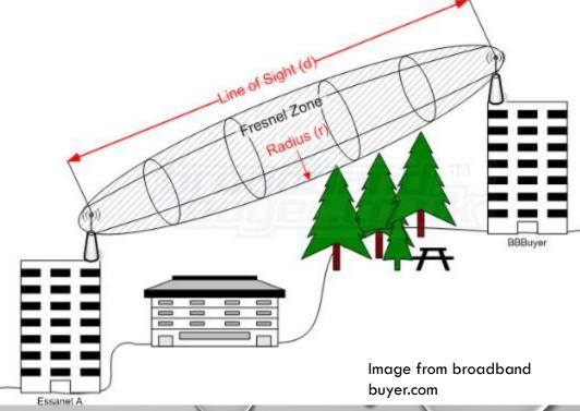
Fresnel Zone in Feet Link distance between antennas (d) in Miles Link frequency (f) in GHz
