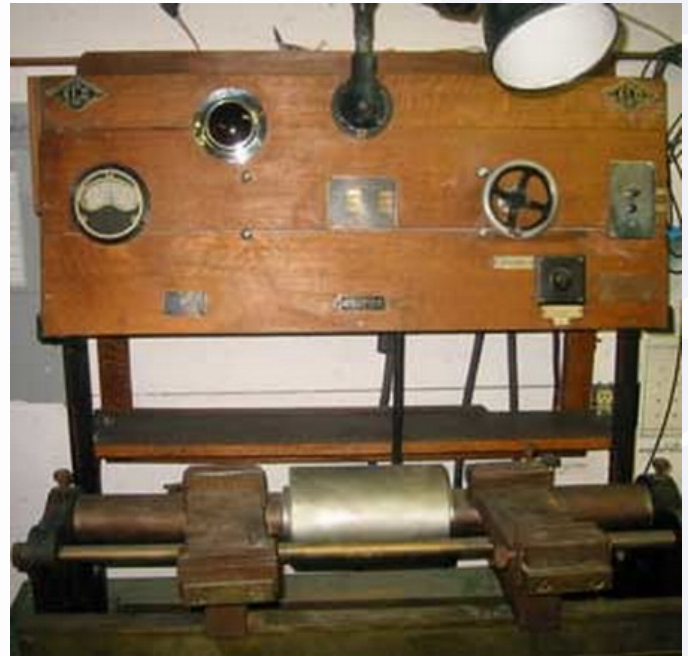
The image shows a 1928 Electyro-Magnetic Steel Testing Device (MPI) made by the Equipment and Engineering Company Ltd. (ECO) of Strand, England. Photo Courtesy of NDT-ed.org
