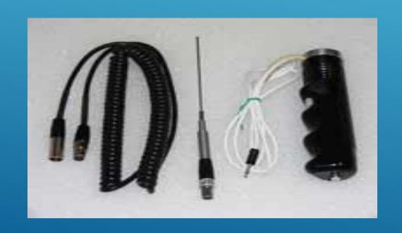
ACCURACY: -40 TO 240 DEGREE F +/- 5% CAN BE CALIBRATED THRU SHORTRIDGE CALIBRATION INTERVAL 12 MONTHS
