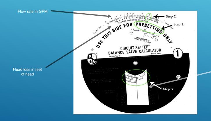
Valve position and valve size
