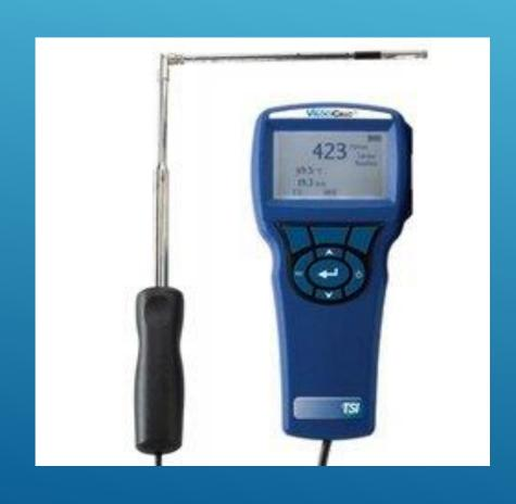
AIR VELOCITY MEASUREMENT 50-3900 FPM +/- 5% OF READING 12 MONTH CALIBRATION
