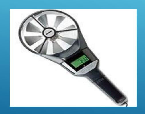
AIR VELOCITY MEASUREMENT 50-3900 FPM +/- 5% OF READING 12 MONTH CALIBRATION
