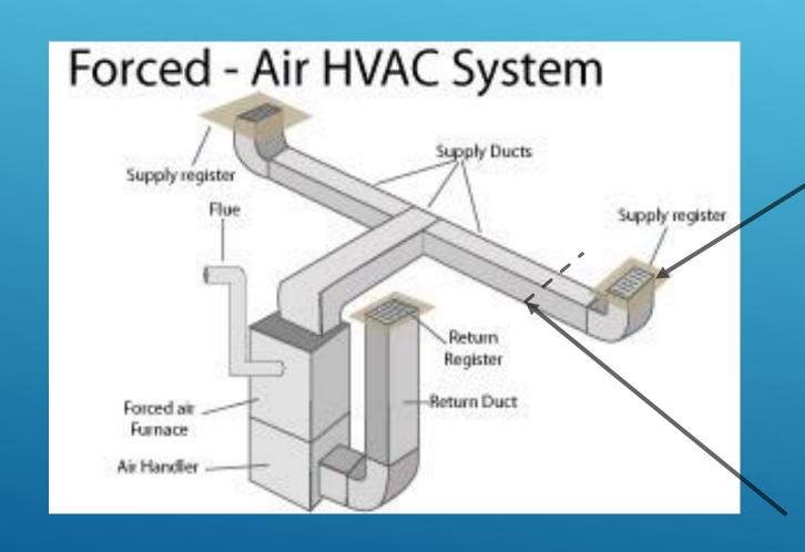
STEP 2: Velocity measured using the appropriate instrument (Shortridge Velgrid or Airfoil, Rotating Vane Anemometer)
