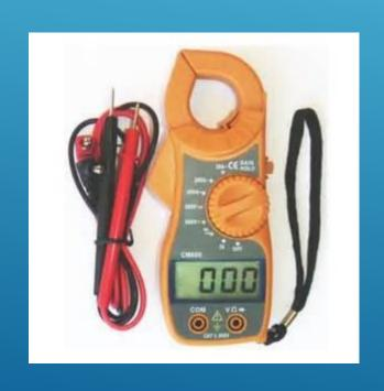
AC VOLTS 0-600 VAC +/- 2% OF READING AMPERES 0-100 AMPERES +/- 2% OF READING 12 MONTH CALIBRATION INTERVAL
