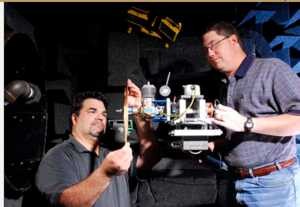
(Top) GTRI senior research engineers Rick Gaeta, left, and Gary Gray display a propeller-dynamometer device developed to test UAV aeroacoustics.
