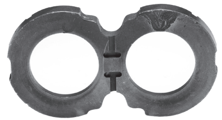
Wear Plate Showing Pitting from Cavitation
